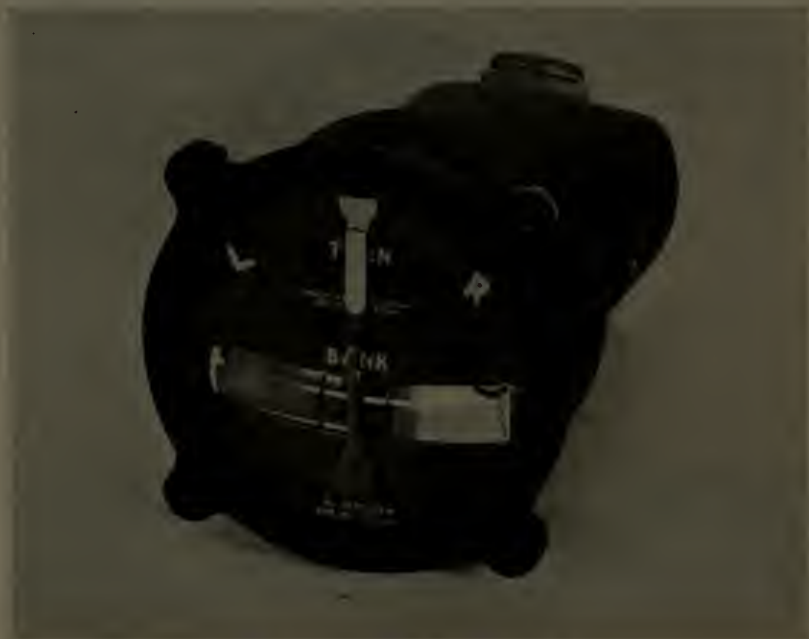
FIGURE 27.—The turn and bank indicator.
